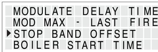
The STOP BAND OFFSET allows us to change the EARLY STOP DEGREES variable. This variable allows the boiler to stop early before it reaches the (setpoint + heat band/2) when the water temperature is moving fast enough to overshoot the top of the band significantly. The default value should be sufficient for most applications. APPLIES: MASTER OR MEMBER
