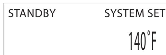
Check that the boiler performs a normal power up and the status screen is displayed. If the firmware did not load correctly the display will remain blank indicating that the control is waiting for a good load. The firmware will need to be reloaded until a normal power up is observed.
