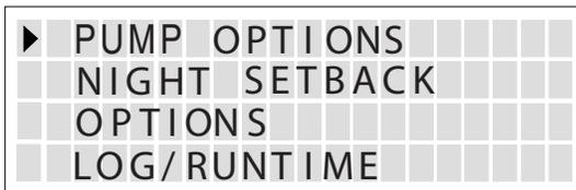
Version 2.1 incorporates the control of a system pump (common system supply pump). A system pump prove dry contact must be placed across the SPARE 3 interlock input. This is the very first interlock, so the H-Net boiler system will not work if this input is open. The on-board relay contacts must be isolated and must only be used to control a motor contactor.
