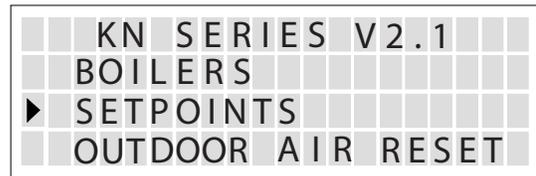
Press the DOWN arrow key to point to SETPOINTS. Then press the SELECT key.
