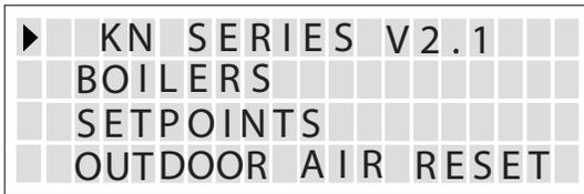
The top line indicates the current firmware (program) revision of the KN boiler's control.
