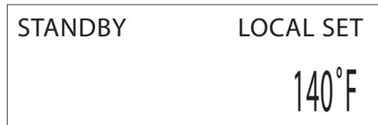
The status screen is actually a menu that is displayed while running or in standby. It is the first screen displayed after the power-up and initialization. It provides all the system runtime status, faults, and calibration settings. You can navigate the status screen by simply pressing on the arrow keys. These keys will allow us to cycle through each screen.
