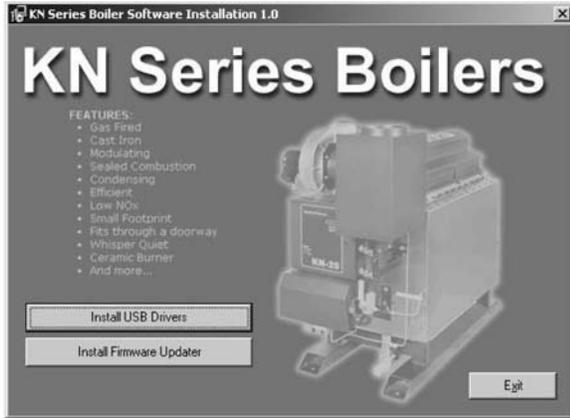
**NOTE: Before beginning the update process, record all setup information. After the Firmware load has completed successfully. You may need to enter setup to verify or restore your settings. The factory ignition settings will remain unchanged.**
