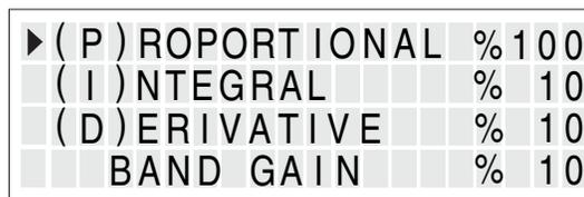
The KN series boiler uses a modified PID algorithm to maintain the water setpoint. The values here may be adjusted **with care** to achieve tight control of the water temperature with changes in load. We recommend that if adjustments are necessary, the Integral value be used primarily and then Derivative value. The default values should be sufficient for most application using the KN series boilers. Remember, you can always load the default values.
