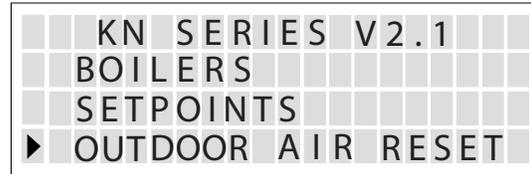
Move the DOWN arrow key to point to OUTDOOR AIR RESET. Press the SELECT key.
