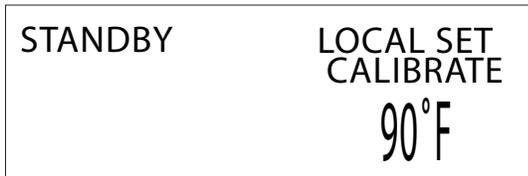
If the status screen does not display CALIBRATE below the setpoint "LOCAL SET" or "SYSTEM SET", check the calibrate switch.
