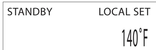
The status screen is the normal display that will be presented during operation and consists of multiple screens. But for now we'll concentrate on how the KN series boiler works using the setup menus. The status screen menus will be reviewed later when we're ready to run.
